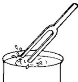
The prongs of a sound producing tuning fork splash water, so they are vibrating.
