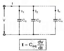
$$C_{eq} = C_1 + C_2 + C_3 + \dots + C_n$$
