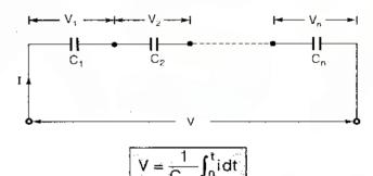
$$\frac{1}{C_{eq}} = \frac{1}{C_1} + \frac{1}{C_2} + \frac{1}{C_3} + \dots + \frac{1}{C_n}$$
