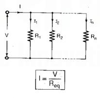
$$\frac{1}{R_{eq}} = \frac{1}{R_1} + \frac{1}{R_2} + \dots + \frac{1}{R_n}$$
