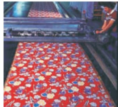
Fig. 17 Roller Printing Machine
