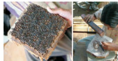
years. Blocks are made of wood with design engraved on the flat surface so that the raised portions of design helps to take the printing paste gets imprinted when stamped. Separate blocks are used for each color. Since block printing is a manual process, it is found to be slow and time consuming. Now-a-days, design is affixed with metal wire which gives a fine print when stamped.
