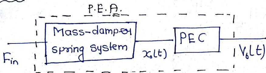
Every accelerometer by default consist of mass damper and spring system
