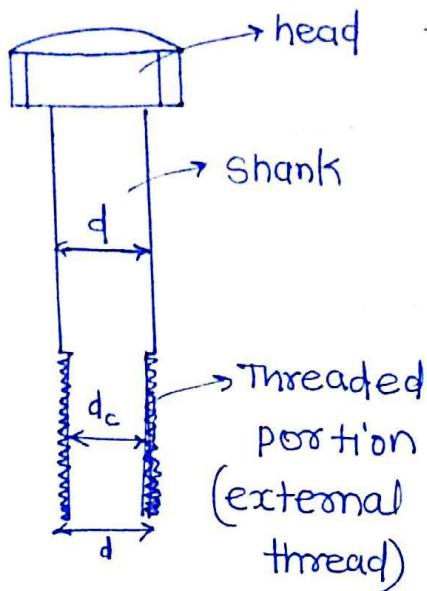
$d = \frac{\text{Major dia}}{\text{Nominal dia}} / \frac{\text{dia of bolt}}{\text{shank dia}}$
