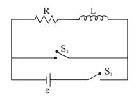
the switch  $S_1$  is closed at time t = 0 and the switch  $S_2$  is kept open. At some later time  $(t_0)$ , the switch  $S_1$  is opened and  $S_2$  is closed. the behaviour of the current I as a function of time 't' is given by: [11 Jan. 2019 II]
