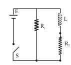
An inductor of inductance L = 400 mH and resistors of resistance  $R_1 = 2\Omega$  and  $R_2 = 2\Omega$  are connected to a battery of emf 12 V as shown in the figure. The internal resistance of the battery is negligible. The switch S is closed at t = 0. The potential drop across L as a function of time is [2009]
