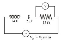
The frequency, at which the voltage across the resistor is maximum, is: [Online April 22, 2013] (a) 902 Hz (b) 143 Hz (c) 23 Hz (d) 345 Hz
