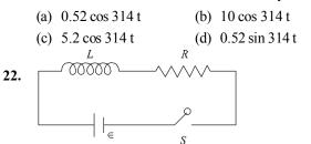
As shown in the figure, a battery of emf  $\in$  is connected to an inductor L and resistance R in series. The switch is closed at t=0. The total charge that flows from the battery, between t=0 and  $t=t_c$  ( $t_c$  is the time constant of the circuit) is:
