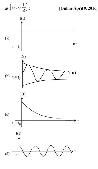
**30.** An inductor (L = 0.03 H) and a resistor (R = 0.15 k $\Omega$ ) are connected in series to a battery of 15V emf in a circuit shown below. The key K<sub>1</sub> has been kept closed for a long time. Then at t = 0, K<sub>1</sub> is opened and key K<sub>2</sub> is closed simultaneously. At t = 1 ms, the current in the circuit will
