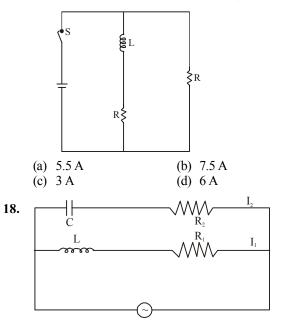
In the above circuit,  $C = \frac{\sqrt{3}}{2} \mu F$ ,  $R_2 = 20 \Omega$ ,  $L = \frac{\sqrt{3}}{10}$  H and  $R_1 = 10 \Omega$ . Current in L-R<sub>1</sub> path is I<sub>1</sub> and in C-R<sub>2</sub> path it is I<sub>2</sub>. The voltage of A.C source is given by,  $V = 200\sqrt{2}$  sin (100 t) volts. The phase difference between I<sub>1</sub> and I<sub>2</sub> is : [12 Jan. 2019 II]
