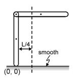
centre of mass does not move in x-direction as  $\Sigma F_x = 0$ .
