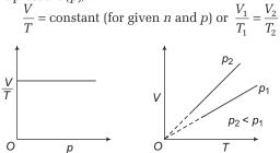
Charles' obtained experimentally that for 1°C change in temperature of a gas, the volume get changed by a fraction of  $\frac{1}{273}$ .
