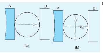
**Fig.E 2.6 (a):** Two magnified views (a) and (b) of a wire showing its perpendicular diameters  $d_1$  and  $d_2$ .  $d_2$  is obtained after the rotating the wire in the clockwise direction through 90°.
