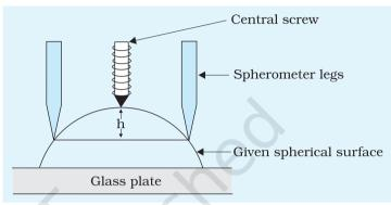
Fig.E 3.4: Measurement of sagitta h
