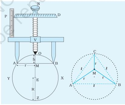
**Fig. E 3.2:** Measurement of radius **Fig. E 3.3:** The base circle of of curvature of a spherical surface
