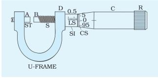
Fig.E 2.2: View of a screw gauge
