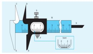
Fig. E 1.1 Vernier Calliper
