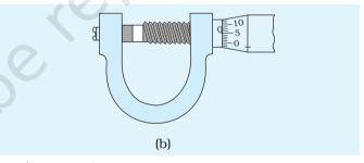
Fig.E 2.4 (b): Showing a negative zero error
