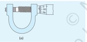
Fig.E 2.4 (a): Showing a positive zero error
