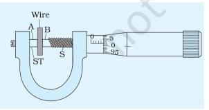
**Fig.E 2.5:** Measuring thickness with a screw guage
