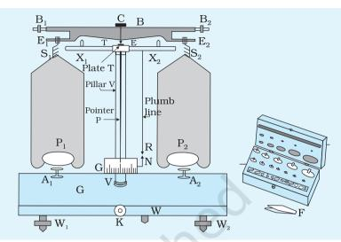
Fig. E 4.2: A physical balance and a weight box
