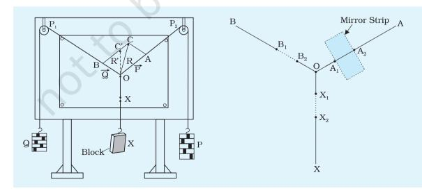
Fig. E 5.1(a): Gravesand's apparatus
