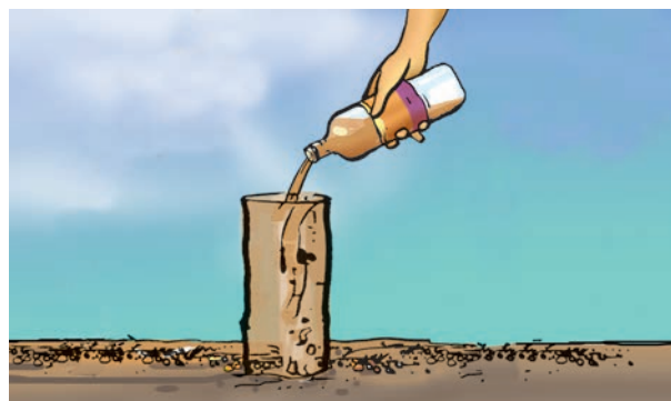
Fig. 9.5 Measuring rate of percolation
