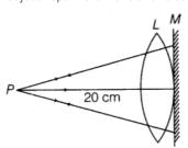
Since, the image is coinciding with the object itself, the rays from the object after refraction from the lens fall normally on the mirror M and form an image coinciding with the object itself. So, the image is formed at the focus of the lens. So, focal length of the lens is 20 cm.
