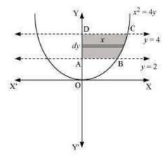
The area of the region bounded by the curve,  $x^2 = 4y$ , y = 2, and y = 4, and the y-axis is the area ABCD.
