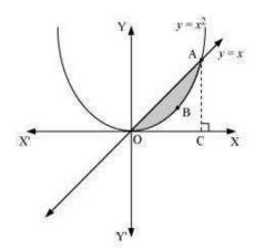
The points of intersection of the curves, y = x and  $y = x^2$ , is A (1, 1). We draw AC perpendicular to x-axis.
