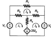
Q.49 The power being dissipated in the 2  $\Omega$  resistor in the following circuit is \_\_\_\_\_ watts.
