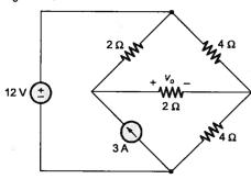
Q.48 The mesh equation for the following circuit are
