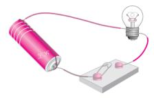
**Ans.** No. The bulb will not glow in this circuit because the switch is open and the circuit is incomplete. Due to this there will be no current flow.
