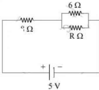
When any resistor is connected parallel to  $6\Omega$  resistance. Then the resistance across that branch ( $6\Omega$  and  $R\Omega$ ) will become less than  $6\Omega$ . i.e., the equivalent resistance of the entire circuit will decrease and hence current will increase. Since,  $V = IR$ , the potential difference across  $8\Omega$  resistor will be larger.
