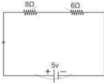
Calculate potential difference across the 8Ω resistor.
