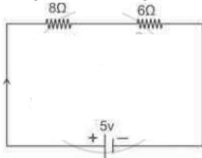
A third resistor is now connected in parallel with 6Ω resistor. Will the potential difference across the 8Ω resistor be larger, smaller, or the same as before? Explain the reason for your answer.
