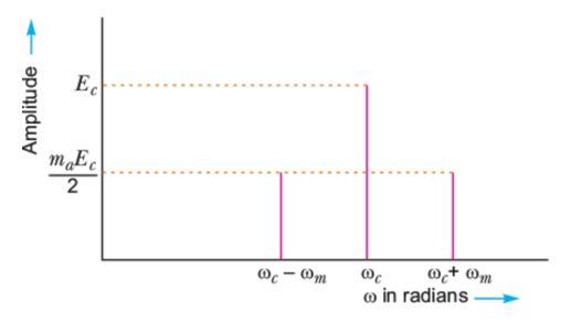
Modulation Index: The ratio of amplitude of modulating signal to the amplitude of carrier wave is called modulation index, i.e., ma =  $\frac{E_m}{E_c}$
