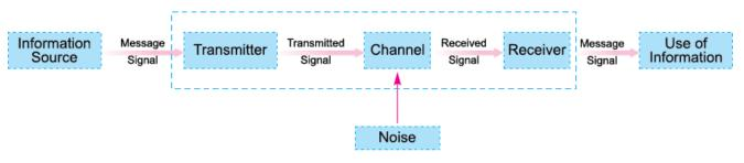
(a) **Transmitter:** A transmitter is an arrangement which processes the incoming message signal so as to make it suitable for transmission through a channel and subsequent reception.
