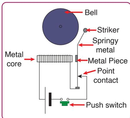
Fig.7.22, Parts of an Electric Bell
