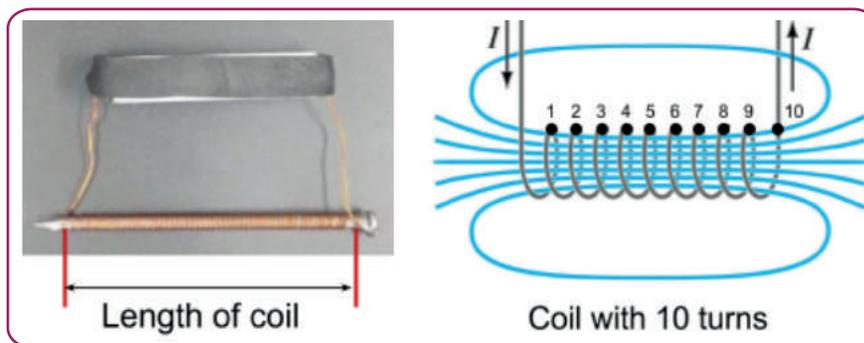
Fig.7.4, How to count number of turns and how to measure length of coil
