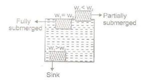
(A) When  $W_1>W_2$ : Weight of the body is greater than the weight of the liquid displaced. This happens when density of the body is greater than density of the liquid.
