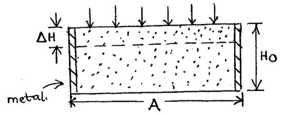
$$m_v = \frac{\Delta V}{V_o \cdot \Delta \sigma'} = \frac{\Delta e}{(1+e_o) \Delta \sigma'}$$
