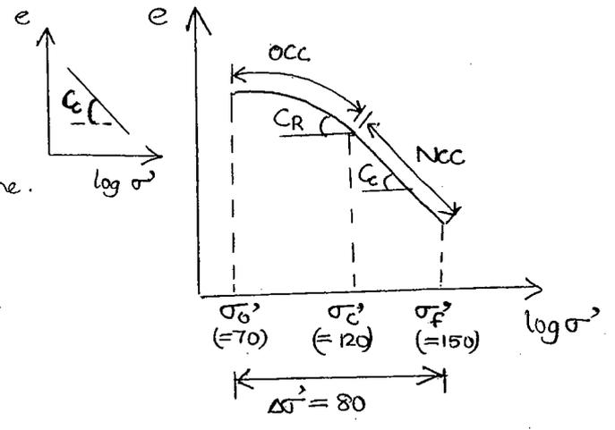
$$\therefore S_f = H_0 \cdot \frac{C_R}{1+e_0} \log_{10} \frac{\sigma'_c}{\sigma'_0} +$$
