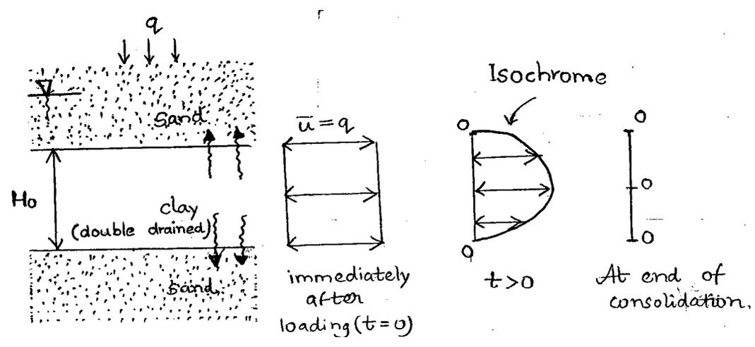
Water tends to escape in vertical direction (to sand has higher permeability), one direction,  $\therefore$  called 1D consolidation.
