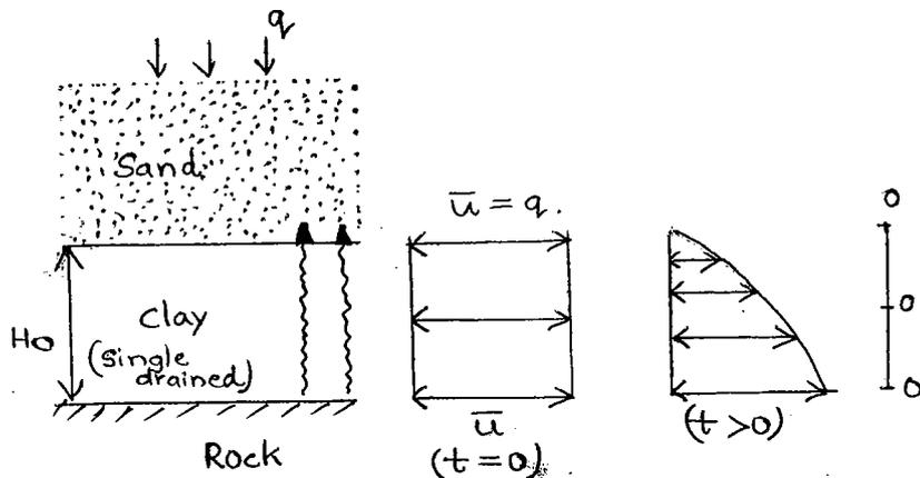
$$\frac{\partial \bar{u}}{\partial t} = \frac{k}{m_v \gamma_w} \frac{\partial^2 \bar{u}}{\partial z^2}$$
