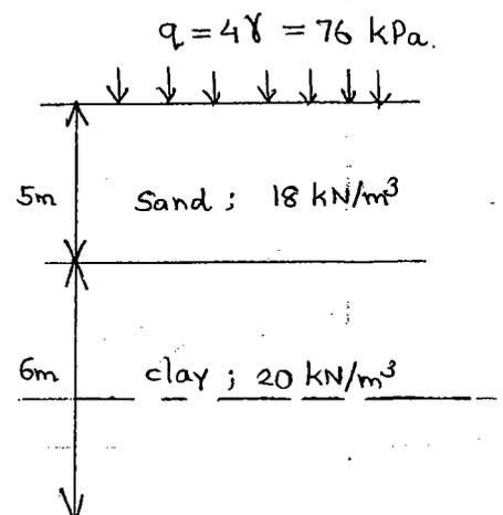
$$\begin{aligned} \sigma' \text{ (immediately after loading)} &= 5\gamma' + 3\delta' \\ &= 5 \times (18 - 10) + 3(20 - 10) \\ &= \underline{\underline{70 \text{ kPa}}} \end{aligned}$$
