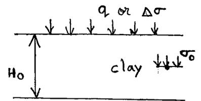
$$(ii) \Delta H \text{ or } S_f = H_o \cdot \frac{C_c}{(1+e_o)} \log_{10} \left( \frac{\sigma'_f}{\sigma'_o} \right)$$
