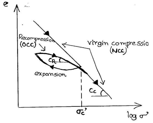
20.  $S_f = H_0 \times \frac{C_c}{1+e_0} \times \log_{10} \left( \frac{\sigma'_f}{\sigma'_0} \right)$
