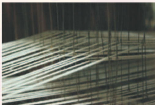
Fig 5.2: Shedding of Warp Sheet
