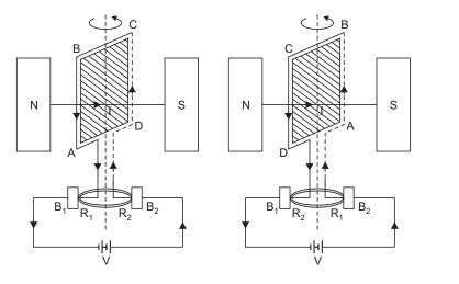
**Working:** As the armature coil is rotated in the mag. field angle  $\theta$  b/w field and normal to the coil changes continuously. An emf is induced in the coil. The direction of induced current is shown in figure.
