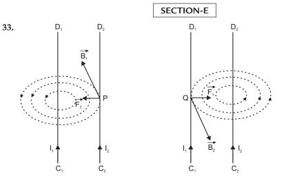
Consider  $C_1 D_1$  and  $C_2 D_2$  two infinite long straight conductors carrying currents  $I_1$  and  $I_2$  in same direction, at a distance r apart held  $||^{el}$  to each other. Mag. field Induction at pt. P on  $C_2 D_2$  due to current  $I_1$  in  $C_1 D_1$ .
