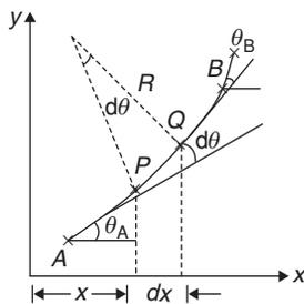
The figure shows elastic curve  $AB$  of an initially straight beam (exaggerated).
