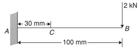
A cantilever beam  $ACB$  is loaded as shown in the above figure. If the flexural rigidity is  $22 \text{ Nm}^2$  determine the slope at point  $C$  using moment area method.
