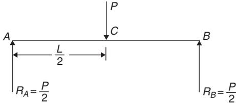
From symmetry, reaction  $R_A = R_B = \frac{P}{2}$
