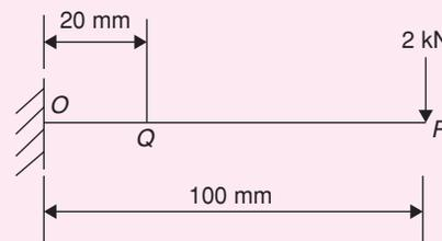
13. A cantilever beam having square cross-section of side  $a$  is subjected to an end load. If  $a$  is increased by 19%, the tip deflection decreases approximately by [2016]
