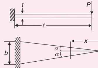
The area moment of inertia about the neutral axis of a cross-section at a distance  $x$  measured from the free end is [2011]
