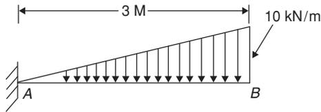
The deflection at point  $B$  for the beam shown in the figure, assuming a flexural rigidity of  $10,000 \text{ kN}\cdot\text{m}^2$  is
