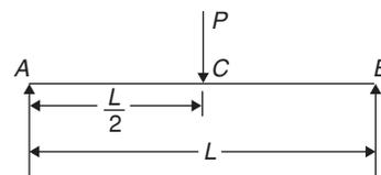
For the simply supported beam loaded as shown in the above figure, determine slope at  $B$  and deflection at  $C$  by area moment method. (Flexural rigidity =  $EI$ )
