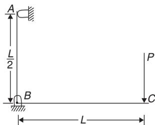
A frame  $ABC$  with 2 arms is hinged at  $B$  and loaded at free end  $C$  as shown in the figure. Each arm of the frame has a flexural rigidity  $EI$ .
