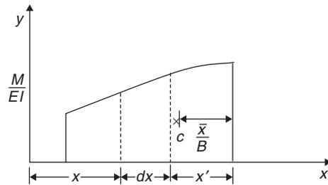
Let  $t_{B/A}$  be the vertical distance of point  $B$  from the tangent to the elastic curve at point  $A$ . This distance is termed as the **tangential deviation** of  $B$  with respect to  $A$ .
