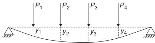
The displacement below any of the points is obtained by differentiating total energy stored in the beam with respect to the
