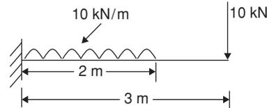
For the cantilever loaded as shown in the figure, the deflection at the end is (Flexural rigidity is given as  $36,000 \text{ kNm}^2$ )
