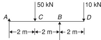
For the beam loaded as shown in the figure, with a flexural rigidity  $36,000 \text{ kNm}^2$ , the deflection at point C is, (Downward deflection +ve)
