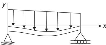
**2. Simply supported beam:** To determine the slope and deflection of the beam at any given point, we first derive the following second order linear differential equation, which governs the elastic curve characterizing the shape of the deformed beam.
