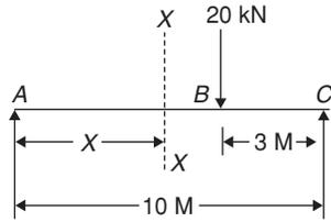
A simply supported beam of 10 m span is loaded as shown in the figure. The deflection at point B is ( $E = 200 \text{ kN/mm}^2 I = 2 \times 10^8 \text{ mm}^4$ )
