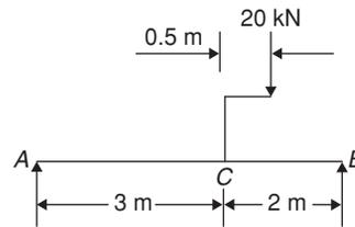
Taking flexural rigidity  $10,000 \text{ kNm}^2$ , the deflection of the beam shown in the figure at point C is
