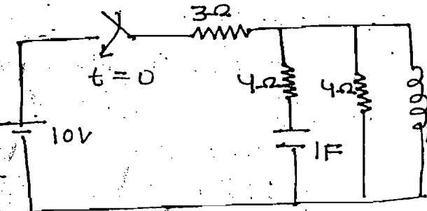
→ In the above ckt. at  $t = 0^-$  capacitor and inductor are uncharged elements.
