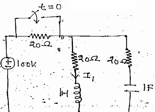
In the above ckt at  $t = 0^-$  for DC source inductor behaves as S.C. and C behaves as an open circuit.
