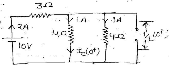
ques:- Find initial voltage and final voltage of the capacitor
