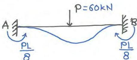
$$M_{FAB} = -\frac{PL}{8} = -\frac{60 \times 6}{8} = -45 \text{ kNm} \quad (-\text{ve becoz anticlockwise})$$
