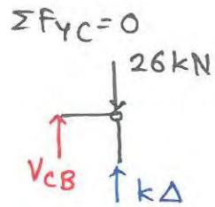
$$V_{CB} + k\Delta - 26 = 0 \quad \dots \dots \text{(ii)}$$
