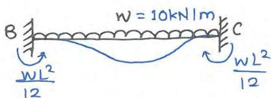
$$M_{FBC} = -\frac{WL^2}{12} = -\frac{10 \times 5^2}{12} = -20.83 \text{ kNm} \quad (-\text{ve becoz anticlockwise})$$
