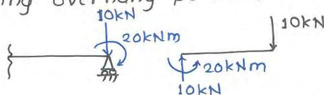
By using modified slope deflection equation for  $M_{BA}$ , unknowns can be reduced to 3 ( $\theta_B, \theta_C, \theta_D$ )
