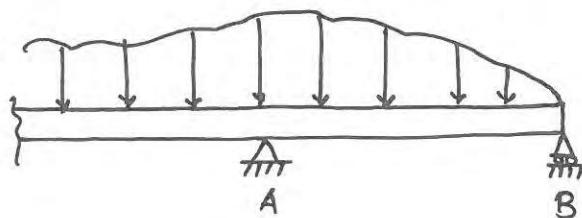
$$M_{AB} = M_{FAB} + \frac{2EI}{L} \left( 2\theta_A + \theta_B - \frac{3\Delta}{L} \right) \quad \dots \text{(i)}$$
