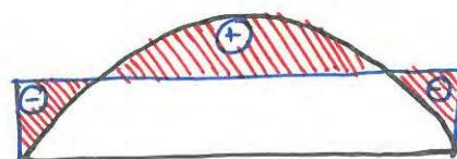
Step I: Draw BMD of span for given loading by considering end condition as pin support and use usual sign convention. (+ve on reference side)
