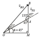
$\frac{v_{BG}}{\sin 135^\circ} = \frac{v_{TG}}{\sin 15^\circ} \implies v_{BG} = 2 \text{ m/s}$
