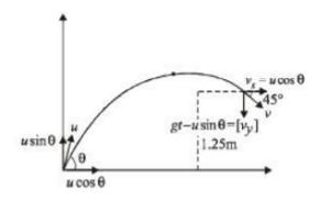
According to question, we have following three conditions. (i) Vertical displacement of stone is 1.25 m.
