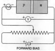
When the p-n junction is forward biased, the depletion layer becomes thin. It is because, the polarity of the external d.c. source opposes the fictitious battery developed across the junction. As a result, the potential drop across the junction decreases making the depletion layer thin. It leads to the low resistance of the junction diode during forward bias.
