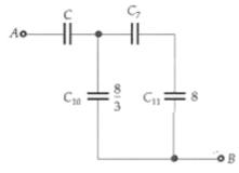
Again, capacitors C<sub>7</sub> and C<sub>11</sub> form a series combination of capacitance C<sub>12</sub> given by
