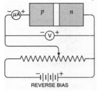
When the p-n junction is reverse biased, the depletion layer becomes thick. It is because, the external d.c. source aids the fictitious battery. It results in the increase of potential drop across the junction and the depletion layer appears thick. Because of the increased thickness of the depletion layer, the p-n junction offers high resistance during reverse bias.
