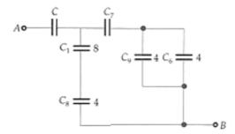
Capacitors C<sub>1</sub> and C<sub>8</sub> form a series combination of capacitance C<sub>10</sub> given by
