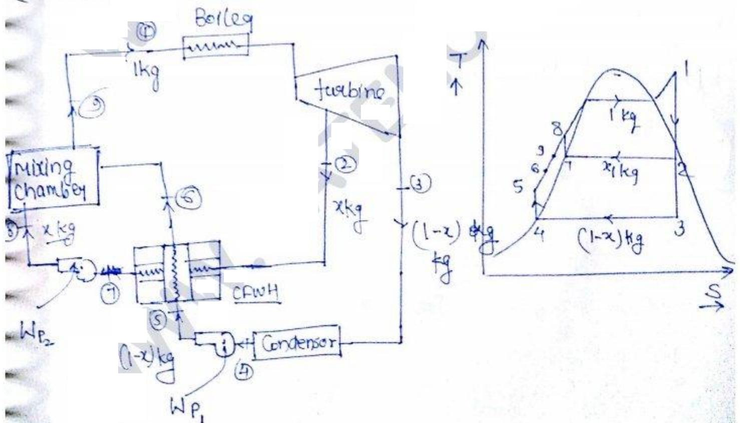
These FWH are proper heat exchanger where heat is transferred from <sup>extracted</sup> steam to <sub>expanded</sub> the feed water without mixing taking place. As the two steam do not mix they can be kept at different pressure
