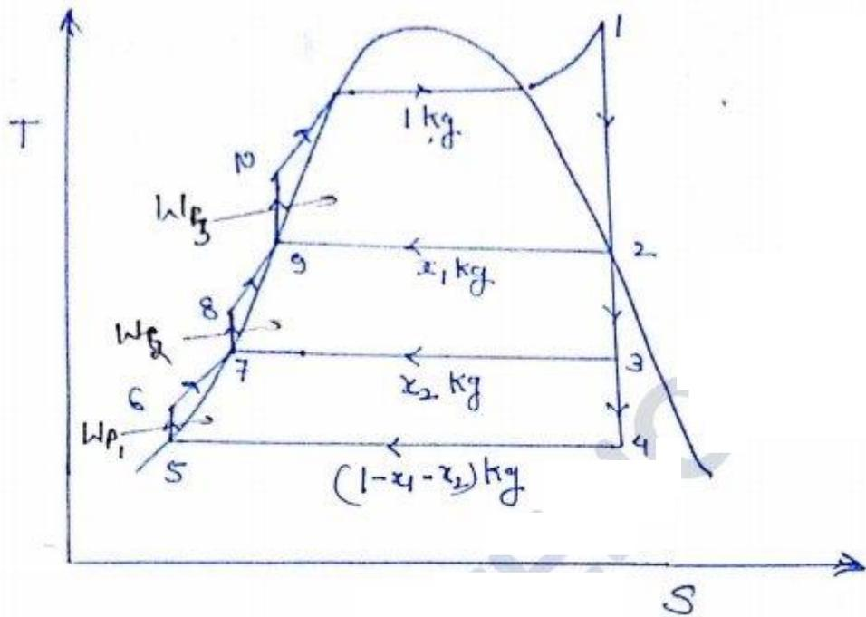
$$W_T = (h_1 - h_2) + (1 - x_1)(h_2 - h_3) + (1 - x_1 - x_2)(h_3 - h_4) \quad \frac{\text{kJ}}{\text{kg}} \text{ of steam}$$
