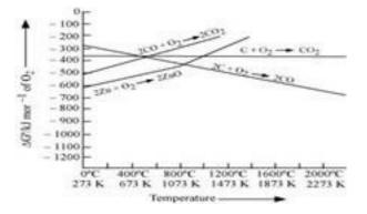
Reduction of ZnO to Zn is usually carried out at 1673 K. From the above figure, it can be observed that above 1073 K, the Gibbs free energy of formation of CO from C and above 1273 K, the Gibbs free energy of formation of  $CO_2$  from C is lesser than the Gibbs free energy of formation of ZnO. Therefore, C can easily reduce ZnO to Zn.
