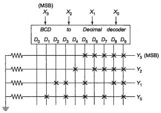
If the coding scheme for  $X_3\,X_2\,X_1\,X_0$  is BCD then find coding scheme for  $Y_3\,Y_2\,Y_1\,Y_0$  .
