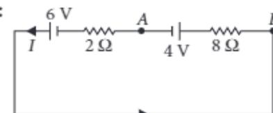
Apply KVL in the given circuit,
