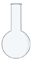
**Flat-bottom flask:** It is a glass container having a spherical bulb with a flattened base and a narrow cylindrical neck. It is used for storing and mixing liquid chemicals and should not be used for heating purposes.
