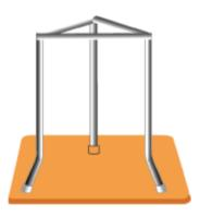
**Asbestos wire gauge:** It is an iron wire mesh with thin asbestos fixed in the middle. It helps in even distribution of heat from the burner to the glass apparatus.
