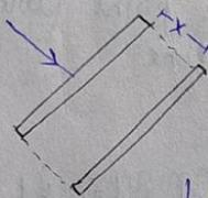
$$\text{Work done} = Fx = P \underbrace{Ax}_{\text{Volume}}$$
