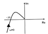
Q.5 The polar plot of frequency response of a linear damped second order system is shown in the figure given. What is the transfer function of this system?
