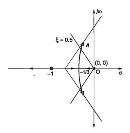
The constant damping ratio line, for  $\xi = 0.5$ , intersects the root locus at point A. The distance from the origin to point A is given as 0.5. The value of K at point A is \_\_\_\_\_.
