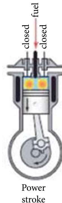
Figure 5.7.1(c) Power Stroke
