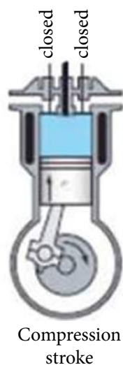
Figure 5.7.1(b) Compression Stroke
