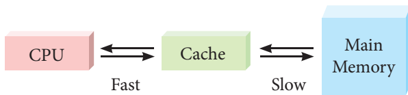
Figure 3.8 Cache Memory Arrangement
