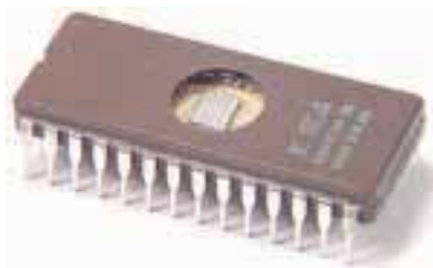
Figure 3.7 Erasable Programmable Read Only Memory
