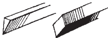
Pointed burin for copper engraving
