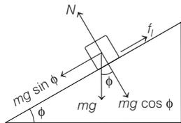
The tangent of the angle of repose is equal to the coefficient of friction.
