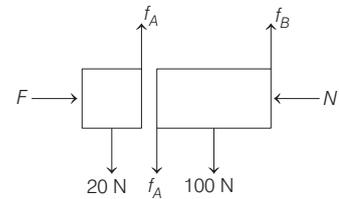
As the blocks are in equilibrium, balance forces are in horizontal and vertical direction.
