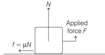
The force of limiting friction  $f_l$  between the surfaces of two bodies is directly proportional to the normal reaction at the point of contact. Mathematically,
