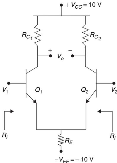
35. The input resistance  $R_i$  seen from each source is
