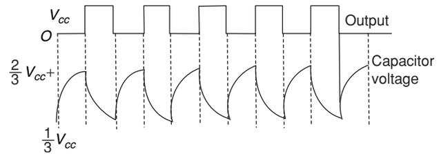
Assume capacitor discharges, when power is switch ON,  $V_{\text{trigger}} = V_{\text{threshold}} = 0$
