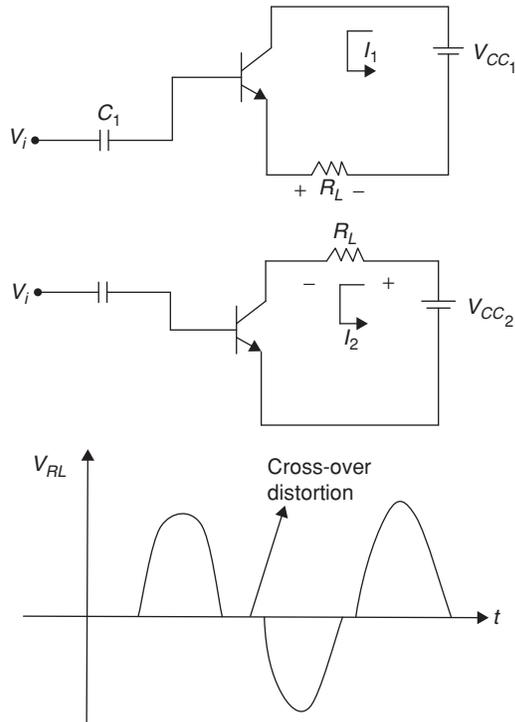
For positive values of sinusoidal input ( $V_i$ )  $Q_1$  conducts and  $Q_2$  is OFF ( $i_2 = 0$ ) so that  $i_1$  is the positive half sine wave.
