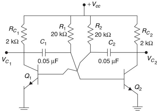
25. The frequency of square wave Output is \_\_\_\_\_.
