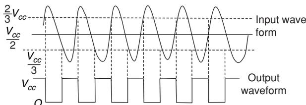
Unlike multivibrators, no frequency division is taking place and frequency of square wave remains same as that of input signal.
