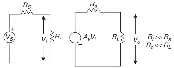
Figure 1 Voltage amplifier
