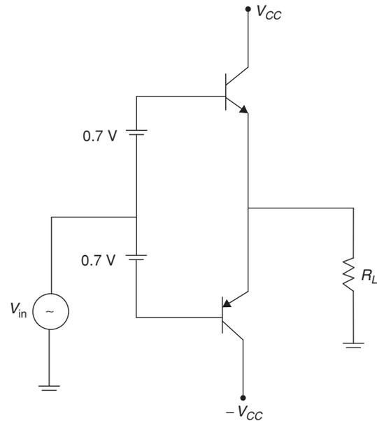
Cross over distortion is eliminated by adding two diodes whose cut in voltages were  $+0.7 \text{ V}$  and  $-0.7 \text{ V}$ .
