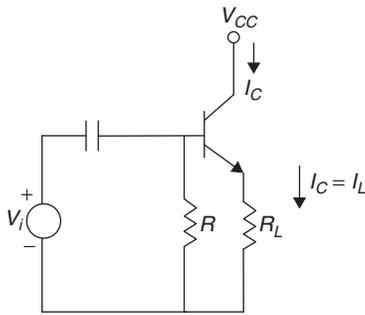
Figure 6 Emitter follower with zero bias operating as class B amplifier
