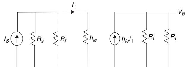
$$A_z = \frac{V_o}{I_s} = \frac{V_o}{I_i} \times \frac{I_i}{I_s} \text{ (Total gain without feedback)}$$
