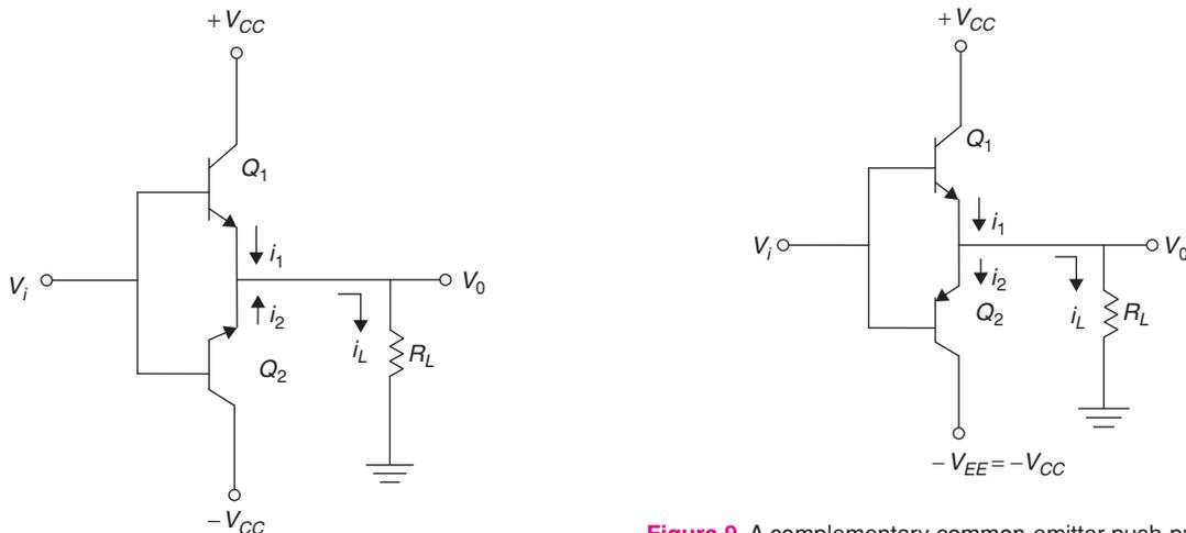
Figure 9 A complementary common-emitter push-pull amplifier
