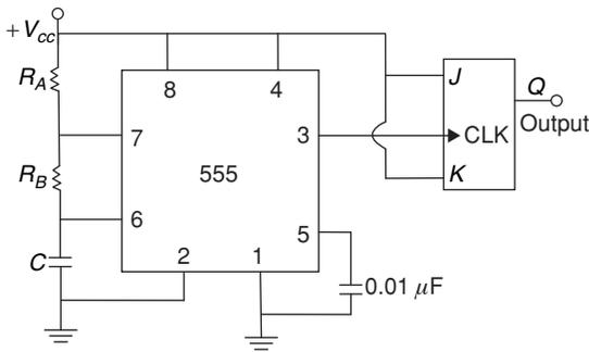
Figure 11 Symmetrical wave form generator.
