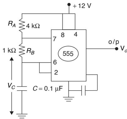
The capacitor voltage  $V_c$  limits are
