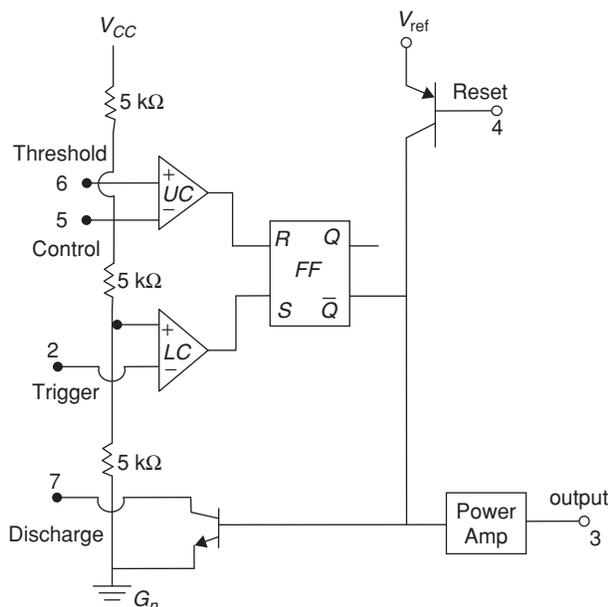
Figure 10 Functional diagram of 555 timer
