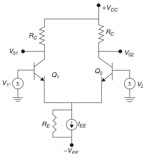
Differential mode voltage gain  $A_{DM} = -g_m R_C$
