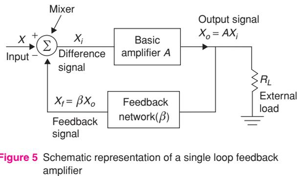
Figure 5 Schematic representation of a single loop feedback amplifier
