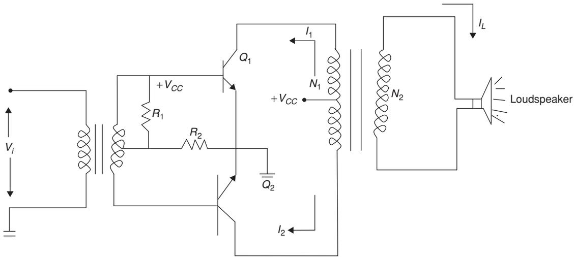
During positive half cycle:  $Q_1$  ON and  $Q_2$  OFF
