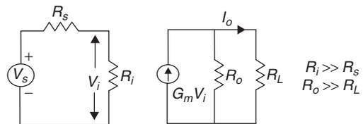
Figure 3 Transconductance amplifier
