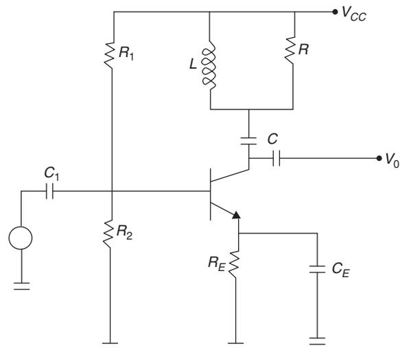
Class C amplifier is used to generate a pulse wave form whose conduction angle is less than  $180^\circ$ . Efficiency of class C amplifier is 90%.
