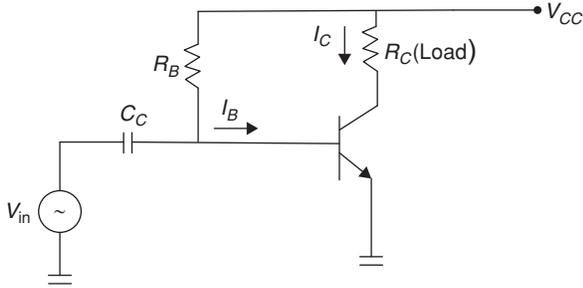
To have maximum output swing, 'Q' point should be located at the middle of the DC load line
