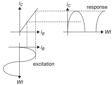
Figure 7 Dynamic transfer characteristic
