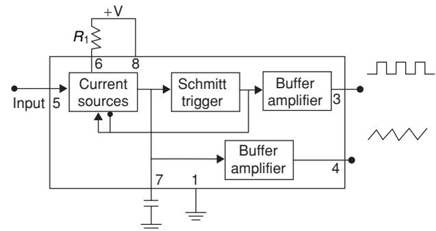
Figure 12 Block diagram. of 566
