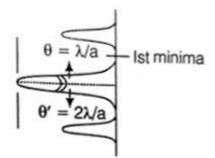
So, angular size of central maxima is  $= 2\left(\frac{\lambda}{a}\right) = \frac{2\lambda}{a}$
