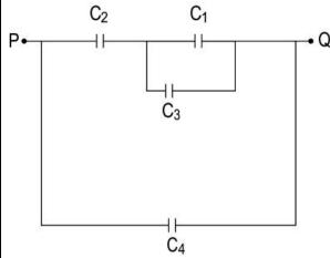
$C_1$  and  $C_3$  are in parallel.
