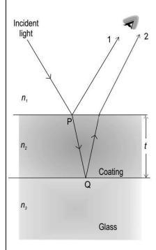
Reflected light undergoes a 180° phase shift when it falls on a denser medium from a rarer medium and no phase shift when it falls on a rarer medium from a denser medium. (Note: The thickness of coating is much less than the glass.)
