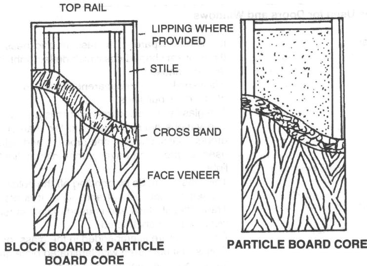
Fig. 15.11: Particle Board
