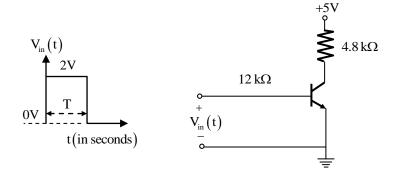
For the input  $V_{in}(t)$  as shown in the figure, the transistor switches between the cut-off and saturation regions of operation, when T is large. Assume collector-to-emitter voltage saturation  $V_{CE(sat)} = 0.2V$  and base-to-emitter voltage  $V_{BE} = 0.7V$ . The minimum value of the common-base current gain ( $\alpha$ ) of the transistor for the switching should be \_\_\_\_\_.
