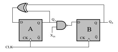
Assume that  $X_{1N}$  is held at a constant logic level throughout the operation of the FSM. When the FSM is initialized to the state  $Q_A Q_B = 00$  and clocked, after a few clock cycles, it starts cycling through
