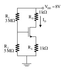
Its threshold voltage  $V_{tn} = 1V$  and its transconductance parameter  $\mu_n C_{ox} \left(\frac{W}{L}\right) = 1 \text{mA}/V^2$ . Neglect channel length modulation and body bias effects. Under these conditions, the drain current I<sub>D</sub> in mA is
