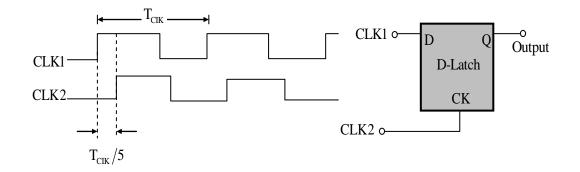
In the figure, the clock signal CLK1 has a 50% duty cycle and CLK2 is a one-fifth period delayed version of CLK1.
