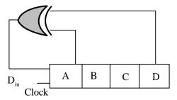
If the present state of the shift register is ABCD = 1101, the number of clock cycles required to reach the state ABCD = 1111 is \_\_\_\_\_.
