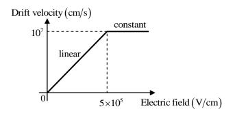
The semiconductor has a uniform electron concentration of  $n = 1 \times 10^{16} \text{ cm}^{-3}$  and electronic charge  $q = 1.6 \times 10^{-19} \text{ C}$ . If a bias of 5V is applied across a 1  $\mu$ m region of this semiconductor, the resulting current density in this region, in kA/cm<sup>2</sup>, is \_\_\_\_\_\_.
