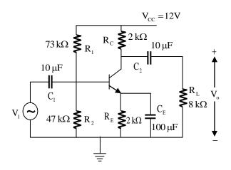
Given that  $V_T = 25 \text{mV}$ ,  $V_{BE} = 0.7 \text{V}$ , and the BJT output resistance  $r_0$  is practically infinite. Under these conditions, the midband voltage gain magnitude  $A_V = |V_0/V_i| V/V$ , is \_\_\_\_\_.
