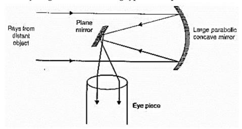
Since a reflecting telescope has mirror objective, the image formed is free from chromatic aberration.
