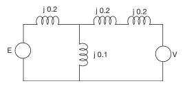
The equivalent reactance during fault X = 0.23Choice (D)
