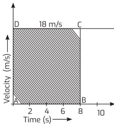
5. From the graph as shown in Q.4, it is clear that the velocity is not changing with time, i.e., acceleration is zero.
