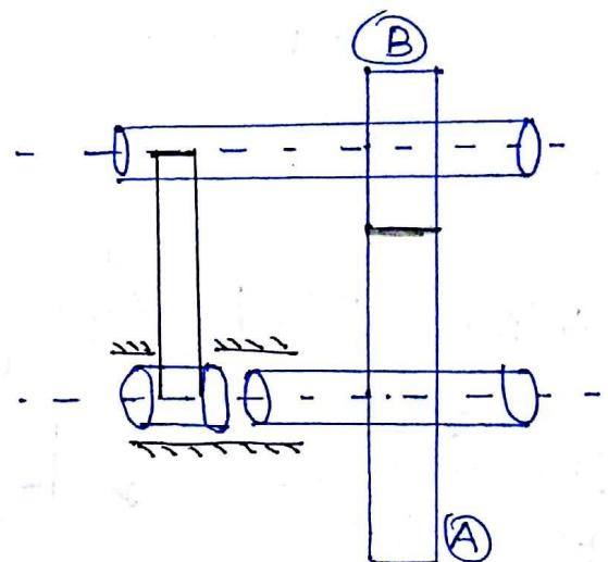
$$\begin{aligned} \text{link } l &= 4 \\ j &= 3 \\ h &= 1 \end{aligned}$$
