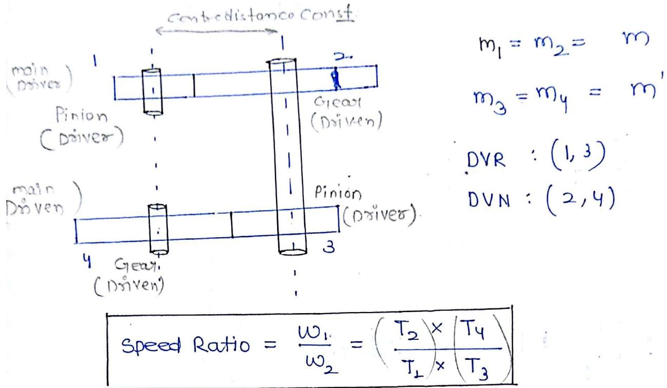
Note:— If in the problem of Reverted Gear train, Speed reduction is Given & same
