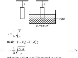
When the object is half immersed in water
