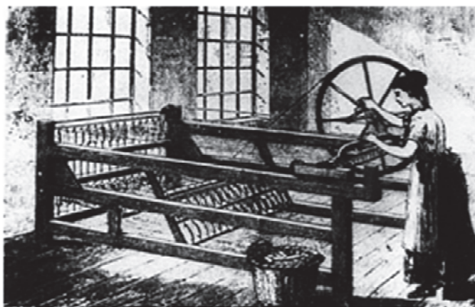
Figure 9.1 The spinning jenny was a new invention to spin cotton faster. It had many spindles in a frame that could be worked by a single worker. What power is being used to run the machine?
