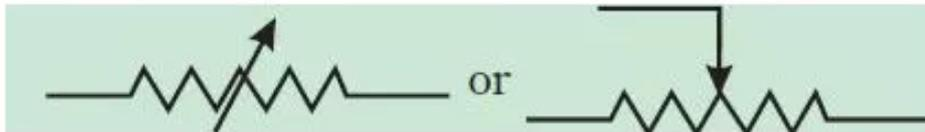
It is used to control the current in the circuit.
