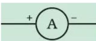
; It is used to measure the current flowing through the circuit.
