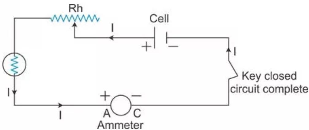
(c) A rheostat is used to control the current in the circuit.
